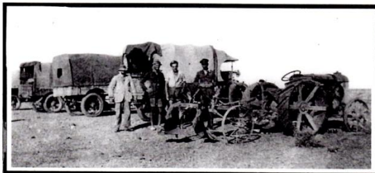
Fordson tractor and double mould board plough used for making the furrow.
